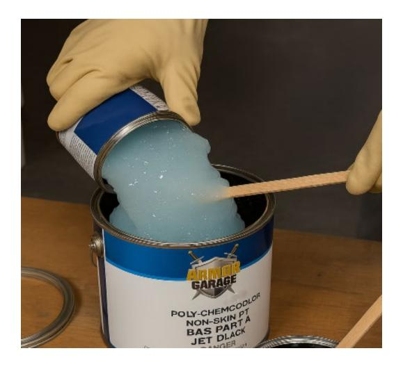
Apply at 40 degrees or warmer. Coverage may vary according to application method and surface porosity. Allow 8 hrs to dry to the touch. Back to service with light traffic within 24hrs depending on temperature and humidity. Allow 48 hours for vehicle traffic.
